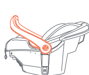
Rebound (Handle MUST be in Rebound position when in vehicle).
