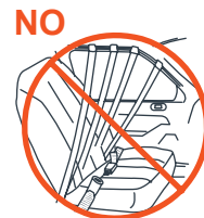
Passive restraints with motorized shoulder belt
